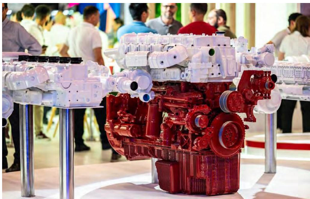
Cummins Helm Engine: Multi-Fuel Proposal Operates on Diesel, Gas or Hydrogen with Head Change.
