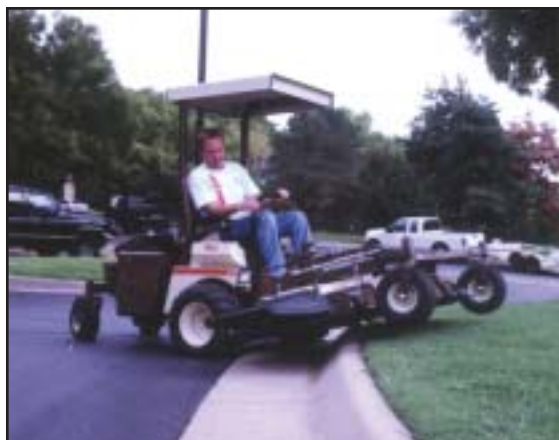
Grasshopper's FrontMount 928D mower features a 72 in. deck and a hydraulic deck lift system, which makes obstacles like curbs less imposing for the operator. The mower is powered by a three-cylinder Kubota liquid-cooled diesel engine rated 28 hp.
